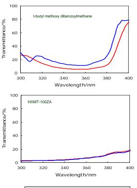
Prior to UV shielding After UV shielding
