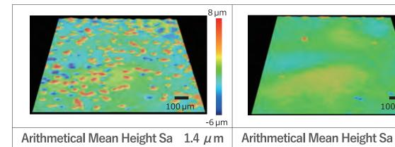
The powder is dispersed into dimethicone to achieve a 10 % concentration, then coat the film using a bar coater. The coating film is then observed under a laser microscope (VK-X 1000).
